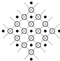
Fig. 6. Intersections of inclined grid (1-5-1 array of points).
