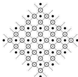
Fig. 12. Intersections of inclined grid (1-7-1 array of points).
